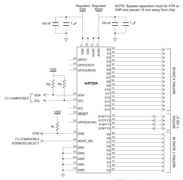
\* NOTE: Y10 to Y13 scan lines may be used as additional X drive lines in extended mode (a  $100\Omega$  resistor must be added to each additional line).
