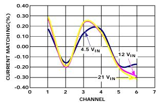
FIGURE 8. CHANNEL-TO-CHANNEL CURRENT MATCHING
