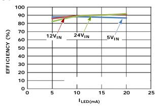
FIGURE 3. EFFICIENCY vs up to 20mA LED CURRENT (100% LED DUTY CYCLE) vs V<sub>IN</sub>
