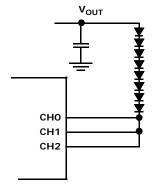
FIGURE 21. GROUPING MULTIPLE CHANNELS FOR HIGH CURRENT APPLICATIONS
