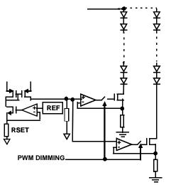
FIGURE 19. SIMPLIFIED CURRENT SOURCE CIRCUIT
