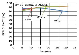
FIGURE 4. EFFICIENCY vs up to 30mA LED CURRENT (100% LED DUTY CYCLE) vs V<sub>IN</sub>
