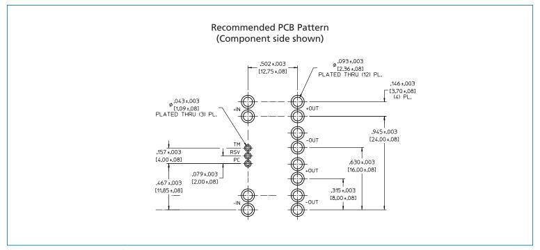
Figure 19 — PCB mounting specifications
