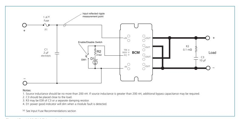
Figure 15 — VI BRICK BCM test circuit
