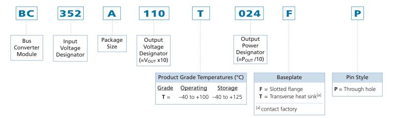
Bus Converter Module BC352A110T024FP vicorpower.com Rev. 1.0 Page 1 of 11
