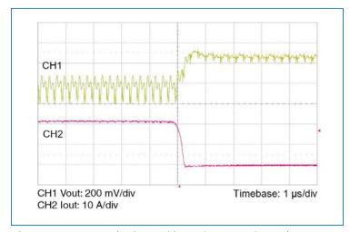
Figure 11 — 21.8-0 A load step with 2  $\mu F$  input capacitor and no output capacitor.
