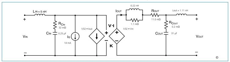
Figure 17 — This model characterizes the AC operation of the VI BRICK bus converter including response to output load or input voltage transients or steady state modulations. The model enables estimates or simulations of input and output voltages under transient conditions, including response to a stepped load with or without external filtering elements.
