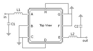
Source/Load Impedance = 50 ohms
