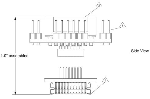
Test points: material- Phosphor Bronze; plating- Sn over  $50\mu^{\text{\tiny "}}$  Ni. Gold flash on contact end.
