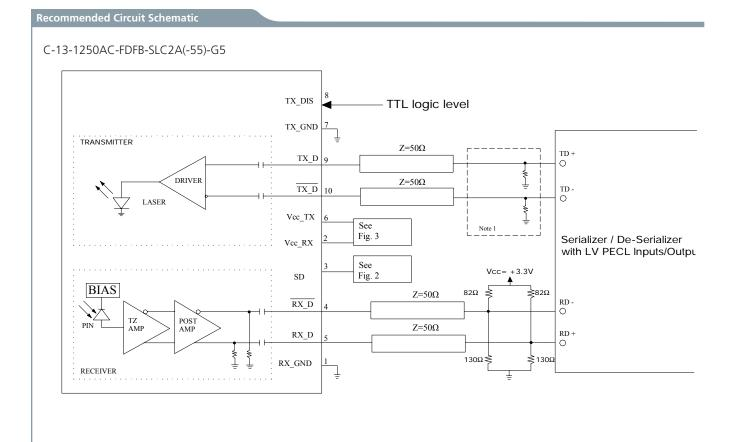
The split-loaded terminations for ECL signals need to be located at the input of devices receiving those ECL signals.
