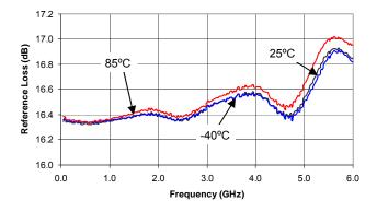
Attenuation - 32 dB Attenuation vs. Frequency
