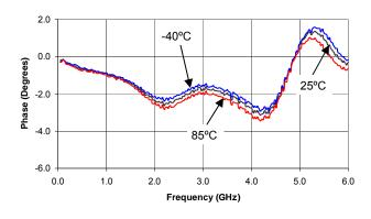
Phase - 16 dB Bit (C2) vs. Frequency Relative to Reference Loss State
