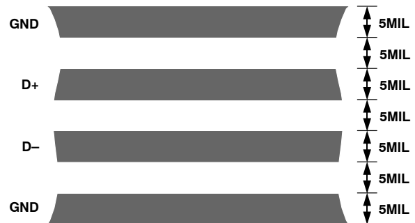
Figure 21. Typical Arrangement of Signal Tracks
