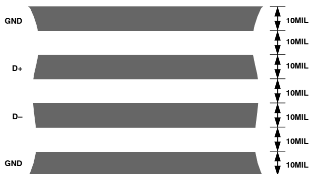
Figure 18. Typical Arrangement of Signal Tracks
