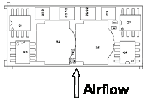
Figure 55. Airflow direction for thermal testing.
