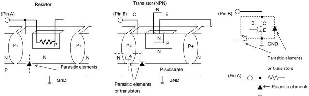
Example of Simple Monolithic IC Architecture
