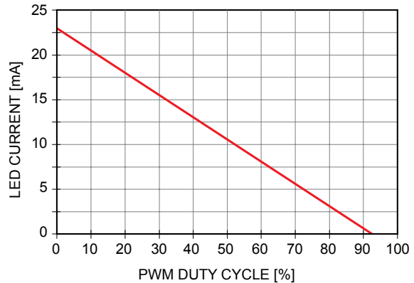
Figure 3. Filtered PWM Dimming [0V to 2.5V]
