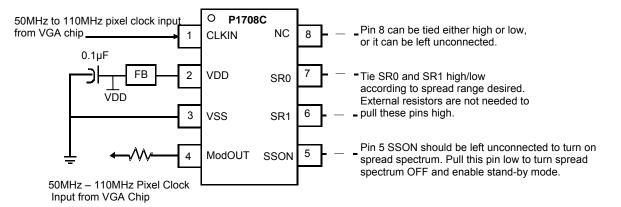
Note: To set the P1708C to standby mode, disable the input clock (pin 1 CLKIN) and pull SSON (pin 5) low. *Refer Standby Mode Selection Table.*
