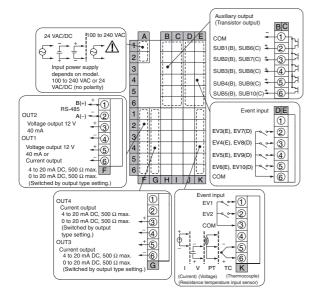
The power supply voltage must be 100 to 240 VAC or 24 VAC/DC for the E5AR-T to comply with CE A Note marking requirements. The power supply voltage must be 100 to 120 VAC or 24 VAC/DC for the E5AR-T to comply with UL requirements.
