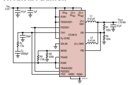
Figure 15. Single, Low Ripple 6A Output
