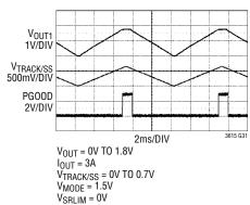
Tracking Up/Down in Forced Continuous Mode, SRLIM Pin Tied to SV<sub>IN</sub>
