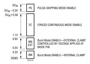
Figure 1. Mode Selection Voltage
