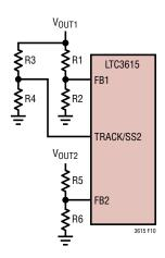
Figure 10. Set for Coincidentally Tracking (R3 = R5, R4 = R6)
