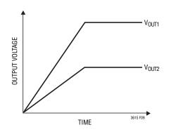
Figure 9. Ratiometric Start-Up Tracking
