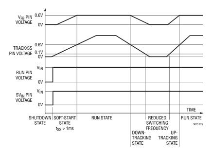
Figure 13. Tracking if  $V_{SRLIM}$  Is Low
