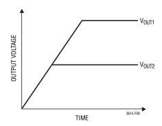
Figure 8. Coincident Start-Up Tracking
