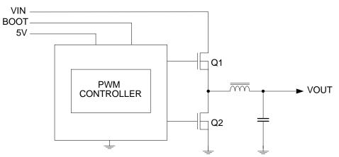
Figure 2: Simplified power system diagram
