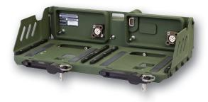
The RF-7800M-AD250 Dual Channel Adapter Plate interfaces up to two JTEL-certified Software Communications Architecture (SCA) AN/PRC-117G(V)1(C) radios to an AM-7588 power amplifier (PA). The adapter allows existing installations of the AN/VRC-103 to update to dual channel JTRS-level multiband and wideband vehicular capabilities, while maintaining the legacy capabilities of traditional multiband vehicular radio systems.
