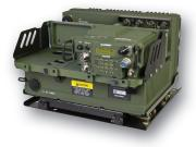
The adapter plate supports single and dual channel operation, allowing existing AM-7588 installations to upgrade to the JTEL- certified Software Communications Architecture (SCA) of the AN/PRC-117G(V)1(C). This upgrade provides JTRS-level multiband and wideband vehicular capabilities while maintaining the legacy capabilities of traditional vehicular radio systems.
