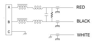
The ZF-1543-3.5B filter has been designed for systems operating under the requirements of MIL-STD-461C and or tempest applications.
