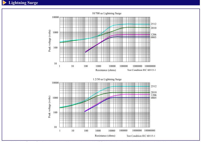
Note: Lightning Surge Resistors are tested in accordance with IEC 60 115-1 using both 1.2/50us and 10/700 pulse.shapes. The limit of acceptance is a shift in resistance of less than 1% from the initial value.
