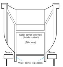
Install a Sensor (or Guide) at each of the four corners indicated by a circle in the following diagram.
