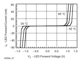
Fig. 1 - LED Forward Current vs.Forward Voltage
