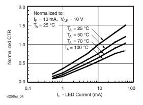
Fig. 4 - Normalized CTR vs.  $I_F$  and  $T_{amb}$
