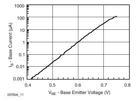
Fig. 11 - Base Emitter Voltage vs. Base Current
