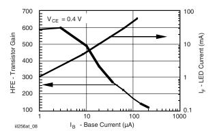
Fig. 8 - Base Current vs.  $I_F$  and  $h_{FE}$
