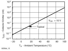
Fig. 12 - Collector-Emitter Leakage Current vs.Temp.
