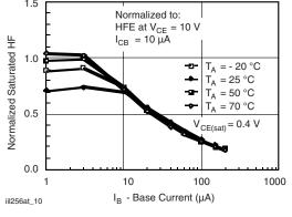
Fig. 10 - Normalized Saturated  $h_{\text{FE}}$  vs. Base Current
