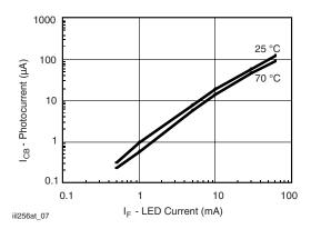
Fig. 7 - Photocurrent vs. LED Current
