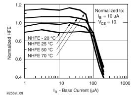
Fig. 9 - Normalized  $h_{\mbox{\scriptsize FE}}$  vs. Base Current and Temp.
