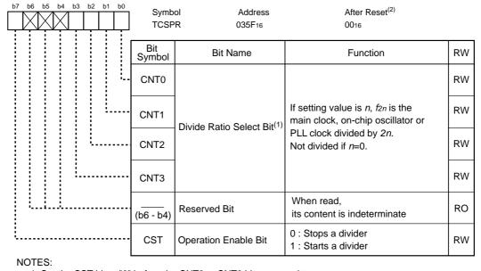
1. Set the CST bit to "0" before the CNT3 to CNT0 bits are rewritten.
