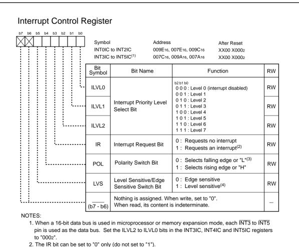
Figure 11.4 Interrupt Control Register (2)
