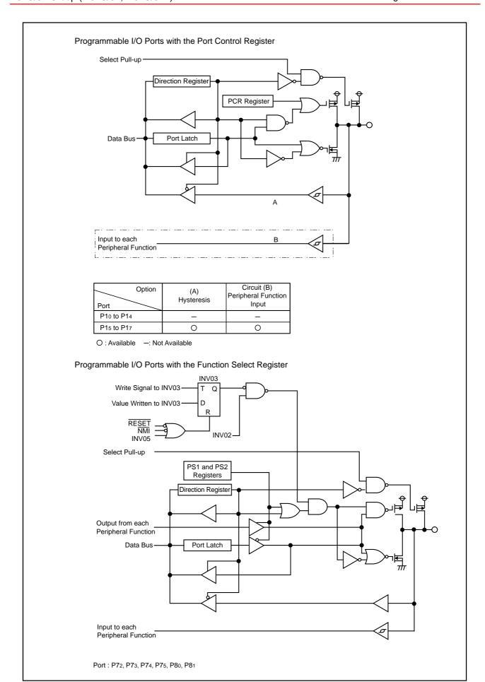
Figure 24.2 Programmable I/O Ports (2)
