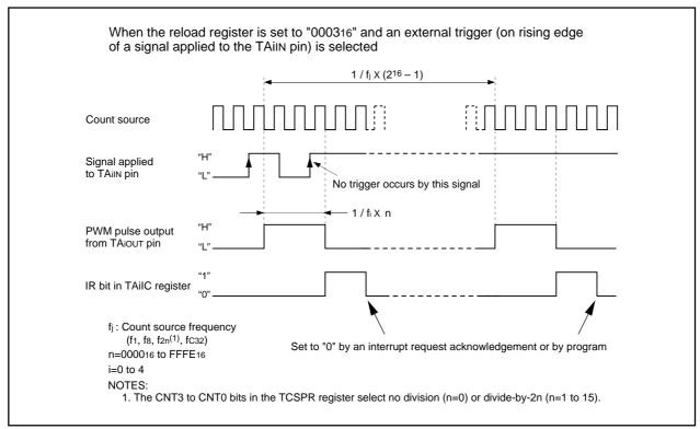
Figure 15.14 16-bit Pulse Width Modulator Operation
