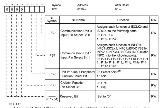
Although AN150 to AN157 can be used when the IPS2 bit is set to "0", power consumption may increase.
