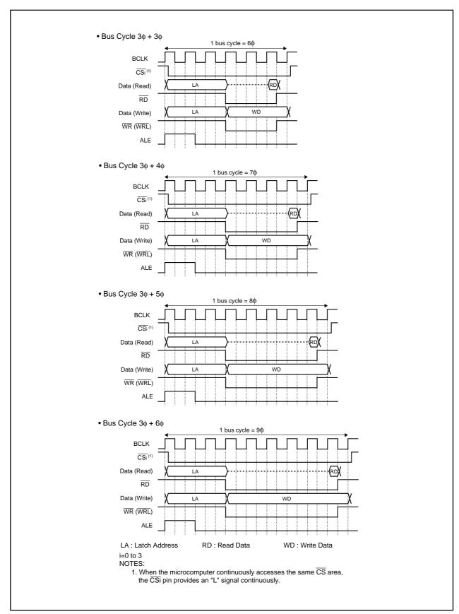
Figure 8.8 Bus Cycle with Multiplexed Bus (2)
