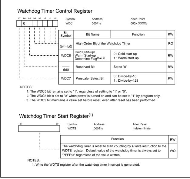
Figure 12.2 WDC Register and WDTS Register
