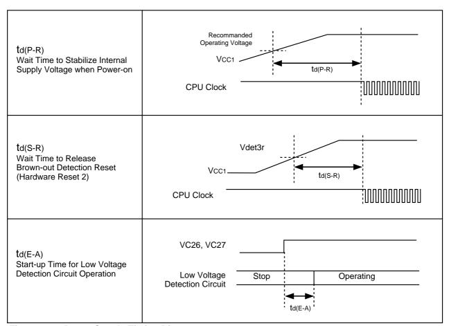
Figure 26.1 Power Supply Timing Diagram
