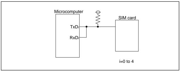
Figure 17.30 SIM Interface Connection
