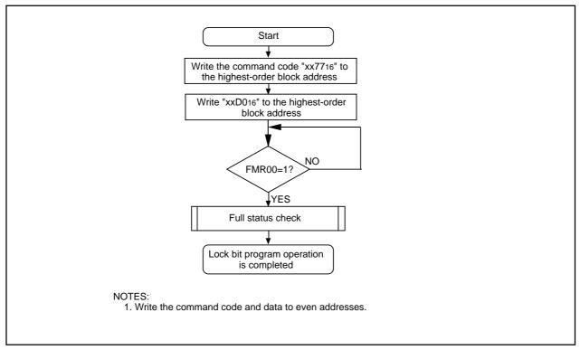
Figure 25.11 Lock Bit Program Command
