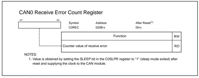
Figure 23.12 COREC Register
