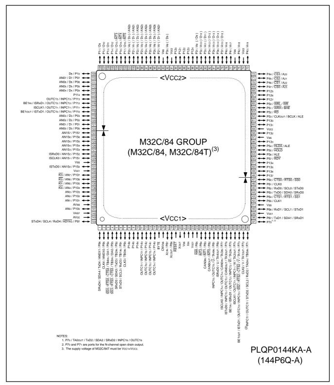
Figure 1.3 Pin Assignment for 144-Pin Package
