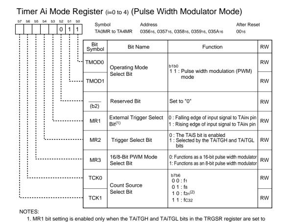
"002" (input to the TAin pin). The MR1 bit can be set to either "0" or "1" when the TAiTGH and TAiTGL bits are set to "012" (TB2 overflow and underflow), "102" (TAi overflow and underflow) or
