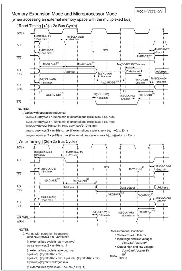
Figure 26.4 Vcc1=Vcc2=5V Timing Diagram (2)
