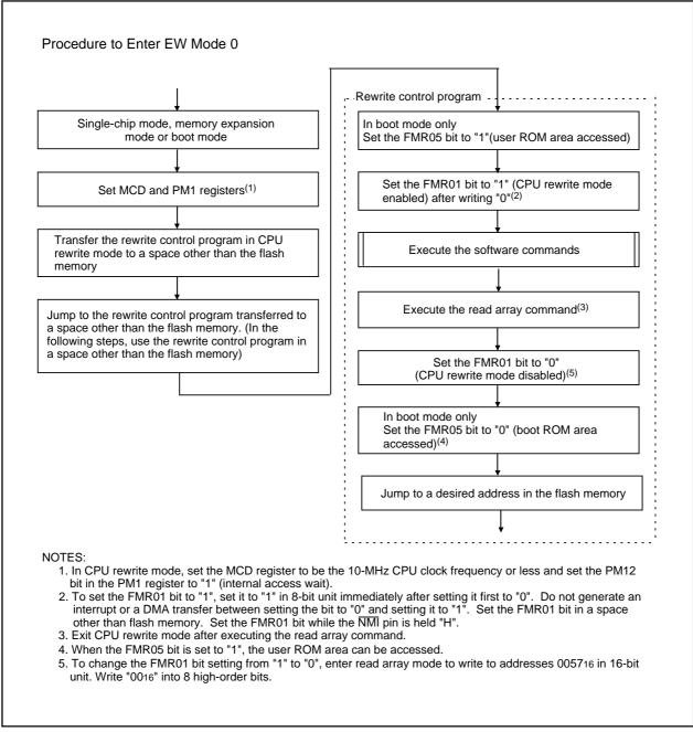
Figure 25.6 How to Enter and Exit EW Mode 0
