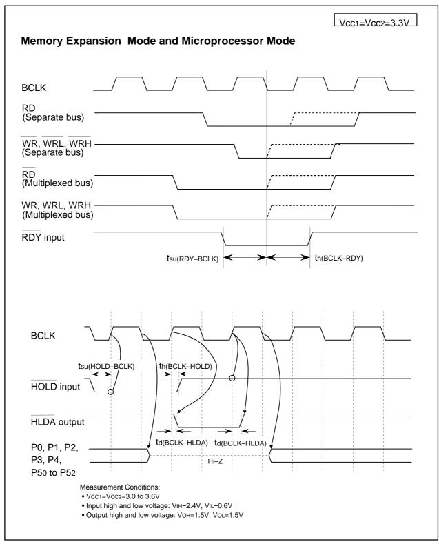
Figure 26.10 Vcc1=Vcc2=3.3V Timing Diagram (4)
