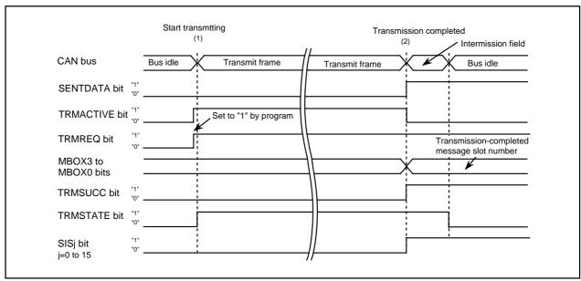
Figure 23.38 Example of CAN Data Frame Transmit Operation
