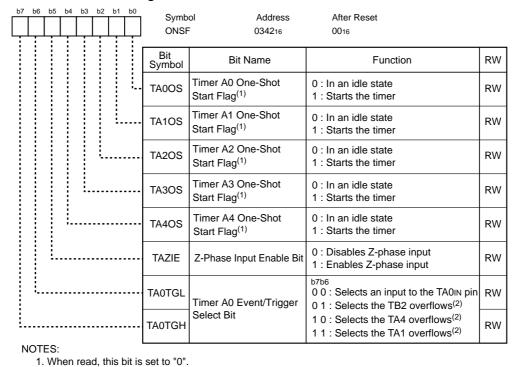
Figure 15.6 UDF Register and ONSF Register
