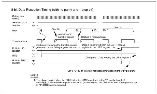
Figure 17.15 Receive Operation
