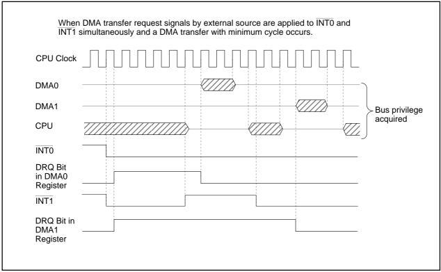
Figure 13.7 DMA Transfer by External Source
