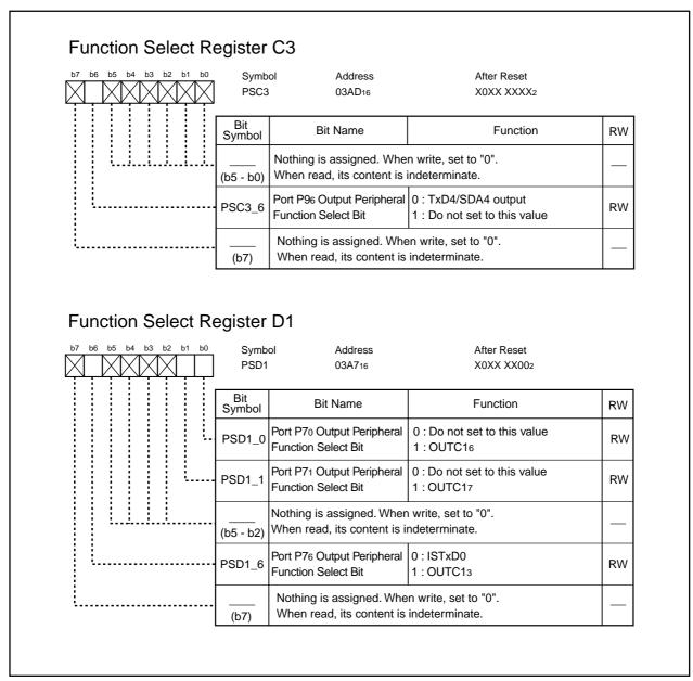
Figure 24.14 PSC3 Register and PSD1 Register
