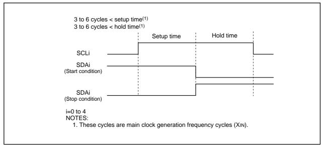
Figure 17.21 Start Condition or Stop Condition Detecting
