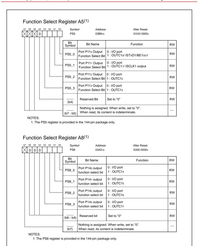
Figure 24.9 PS5 Register and PS8 Register
