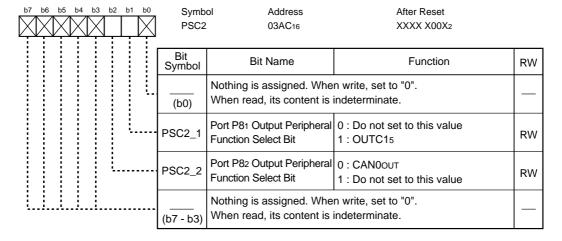
Figure 24.13 PSC Register and PSC2 Register
