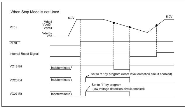
Figure 5.3 Brown-out Detection Reset (Hardware Reset 2)
