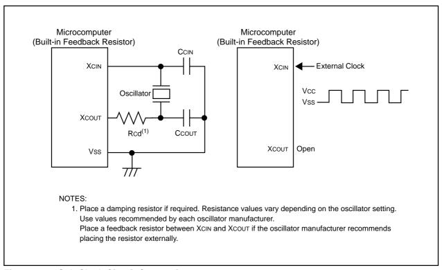
Figure 9.10 Sub Clock Circuit Connection
