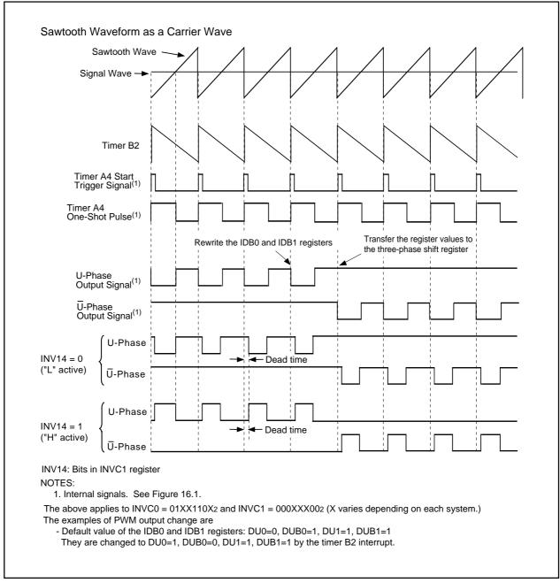
Figure 16.9 Sawtooth Wave Modulation Operation
