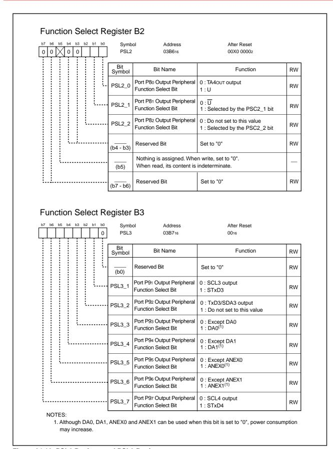
Figure 24.12 PSL2 Register and PSL3 Register
