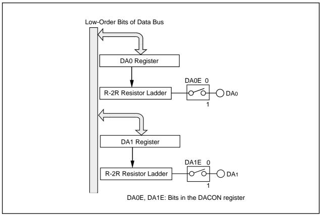
Figure 19.1 D/A Converter
