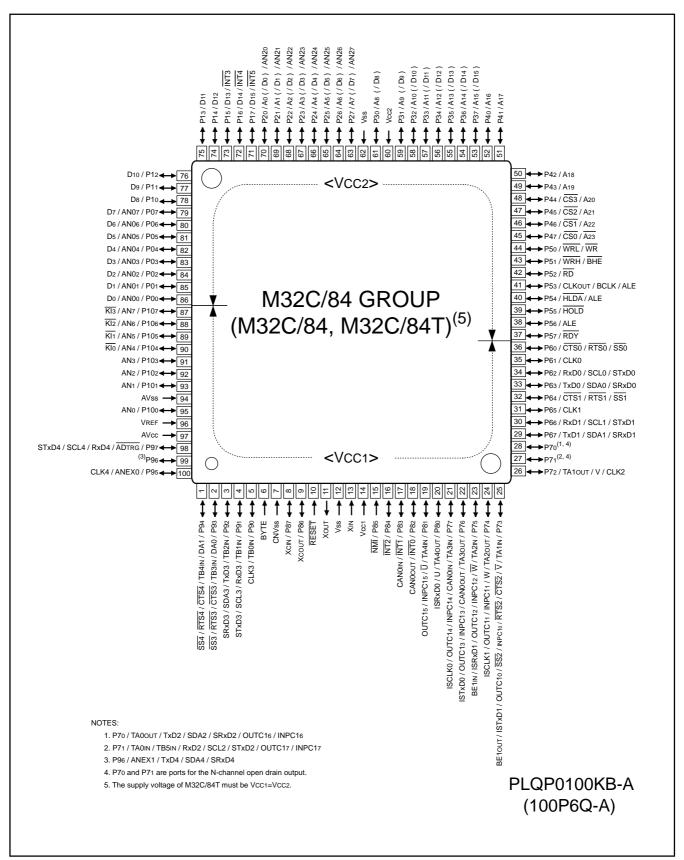
Figure 1.5 Pin Assignment for 100-Pin Package
