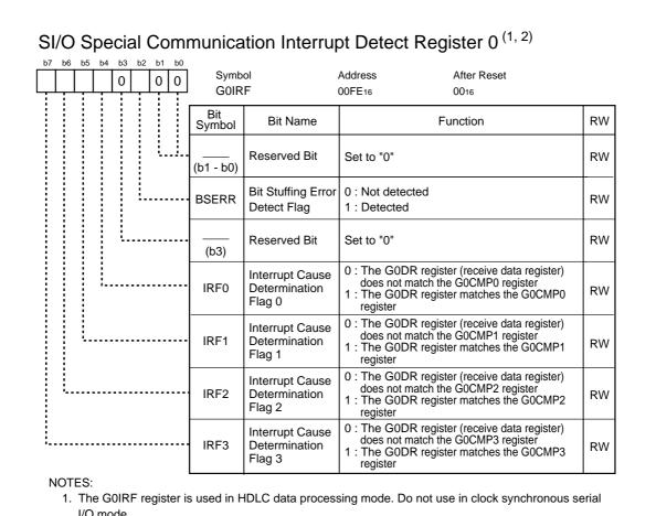
2. The SRTOR bit in the IIO4IR register is set to "1" if the BSERR or IRF0 to IRF3 bit is set to "1".
