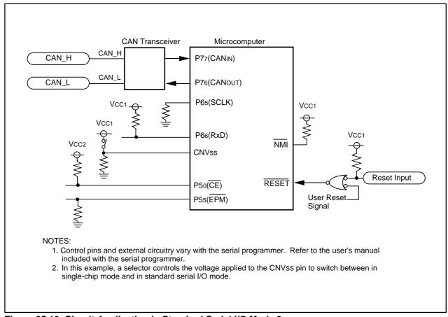
Figure 25.19 Circuit Application in Standard Serial I/O Mode 3
