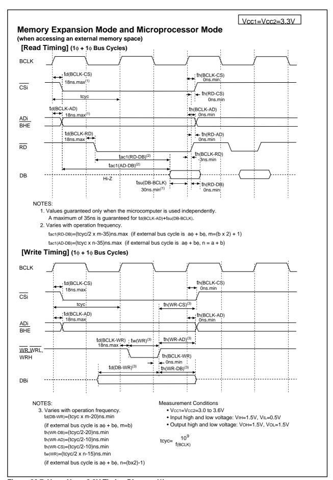
Figure 26.7 Vcc1=Vcc2=3.3V Timing Diagram (1)
