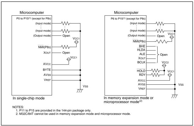
Figure 24.19 Unassigned Pin Handling
