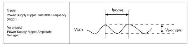
Figure 27.2 Power Supply Fluctuation Timing
