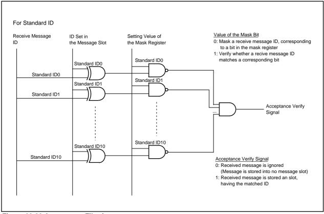
Figure 23.28 Acceptance Filtering
