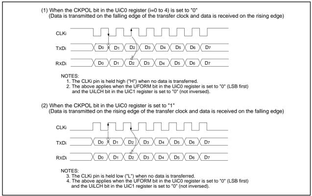
Figure 17.11 Transfer Clock Polarity
