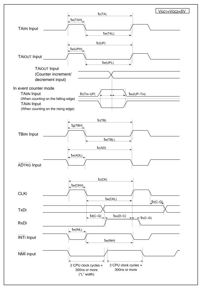
Figure 26.5 VCC1=VCC2=5V Timing Diagram (3)
