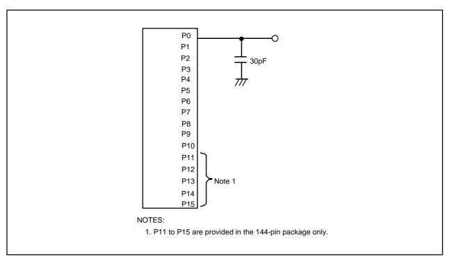
Figure 26.2 P0 to P15 Measurement Circuit
