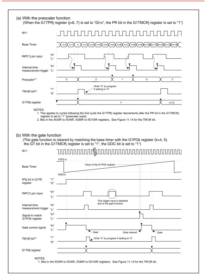
Figure 22.15 Prescaler Function and Gate Function
