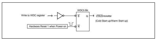
Figure 6.7 Cold Start-up/Warm Start-up Determine Function Block Diagram
