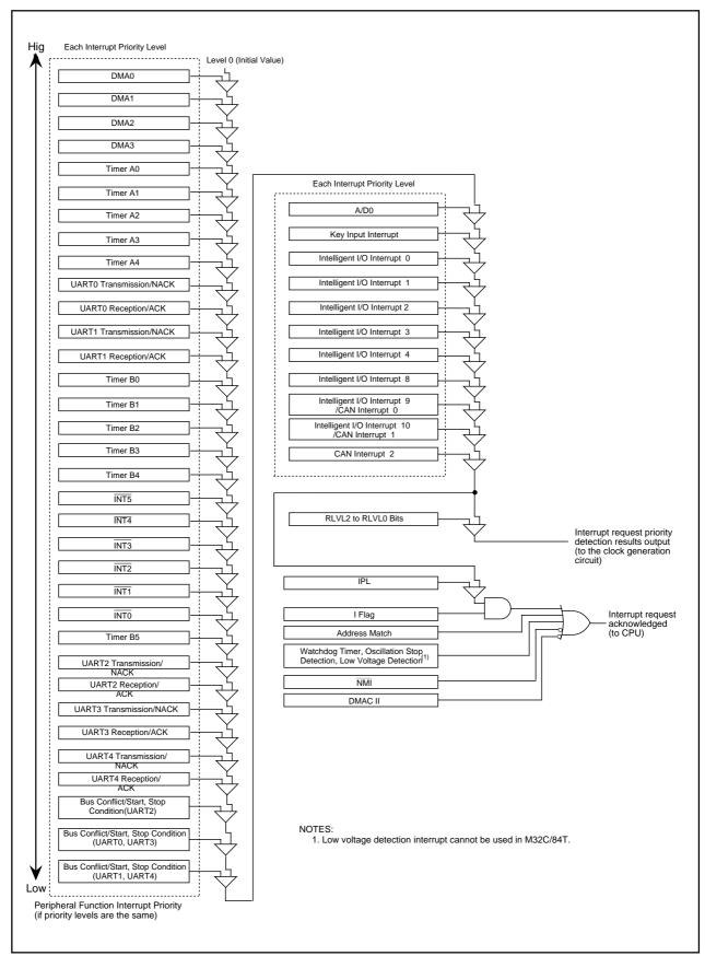
Figure 11.9 Interrupt Priority Level Select Circuit
