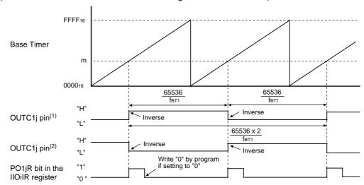
i=0 to 4, 8 to 10; j=0 to 7 m: Setting value of the G1POj register, 000016 to FFFF16
