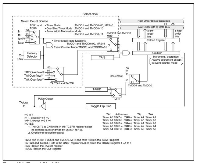
Figure 15.3 Timer A Block Diagram
