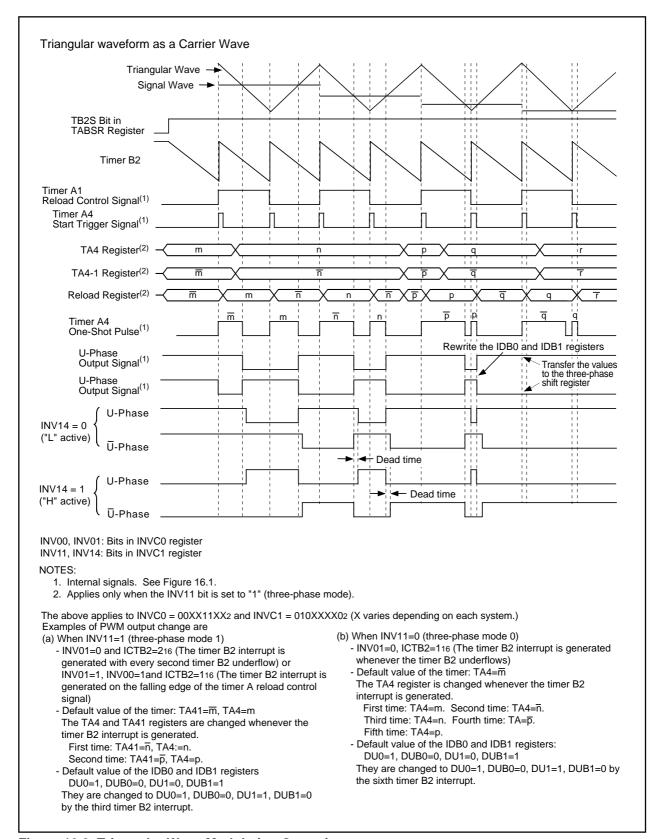
Figure 16.8 Triangular Wave Modulation Operation
