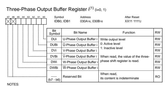
1. Values of the IDB0 and IDB1 registers are transferred to the three-phase output shift register by a transfer trigger.
