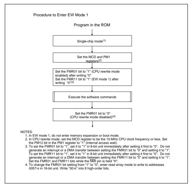
Figure 25.7 How to Enter and Exit EW Mode 1
