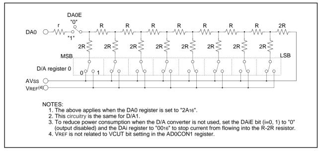
Figure 19.3 D/A Converter Equivalent Circuit
