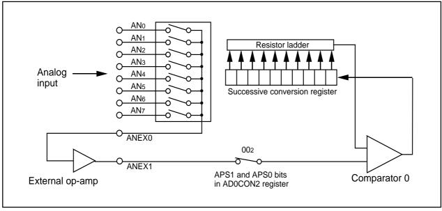
Figure 18.7 External Op-Amp Connection
