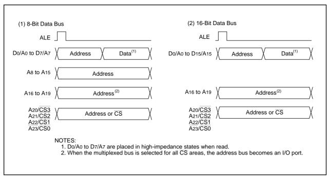
Figure 8.10 ALE Signal and Address/Data Bus
