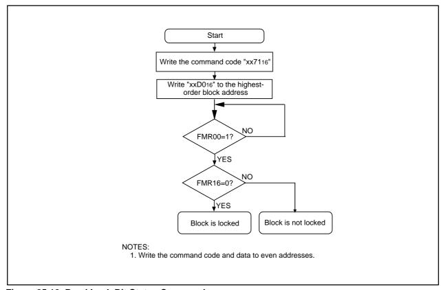
Figure 25.12 Read Lock Bit Status Command
