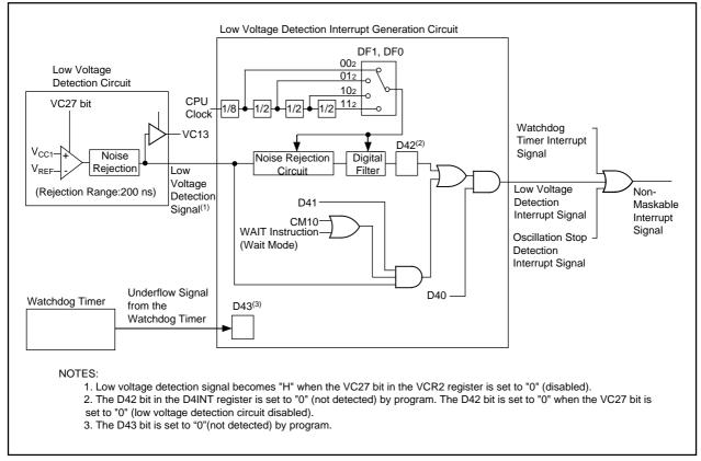
Figure 6.5 Low Voltage Detection Interrupt Generation Circuit
