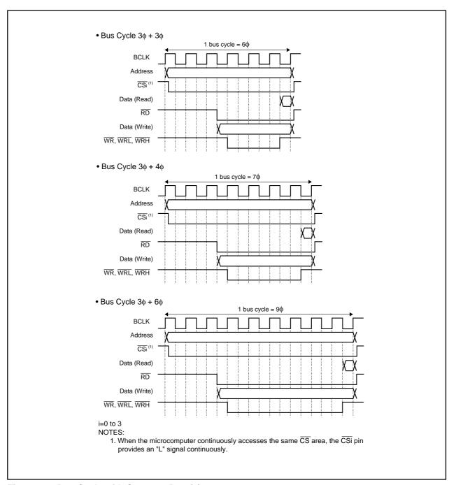
Figure 8.6 Bus Cycle with Separate Bus (3)
