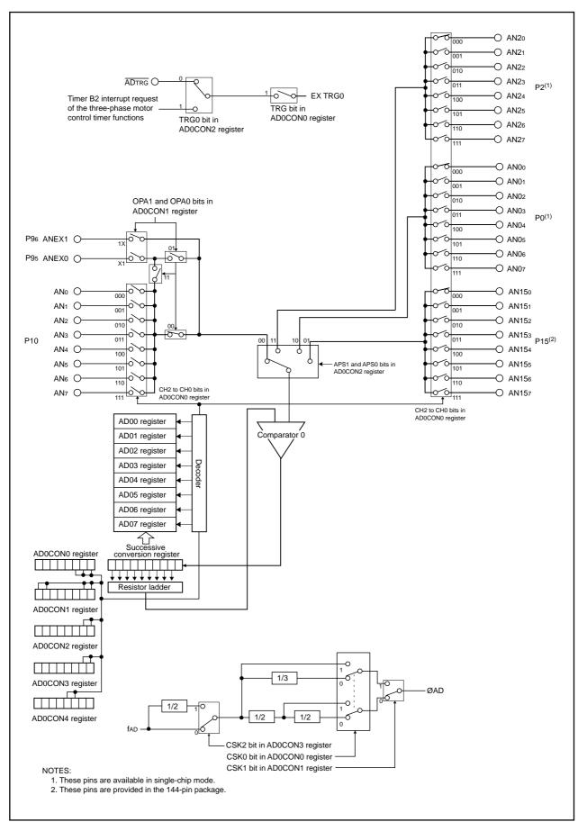
Figure 18.1 A/D Converter Block Diagram
