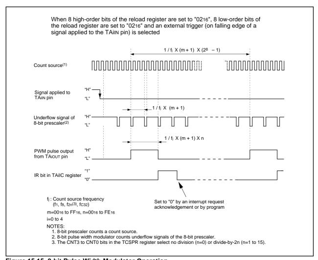
Figure 15.15 8-bit Pulse Width Modulator Operation
