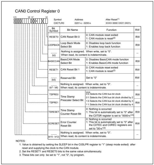
Figure 23.3 C0CTLR0 and C1CTLR0 Registers
