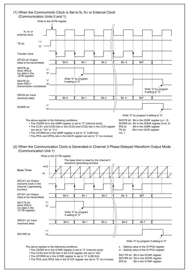
Figure 22.30 Transmit and Receive Operation
