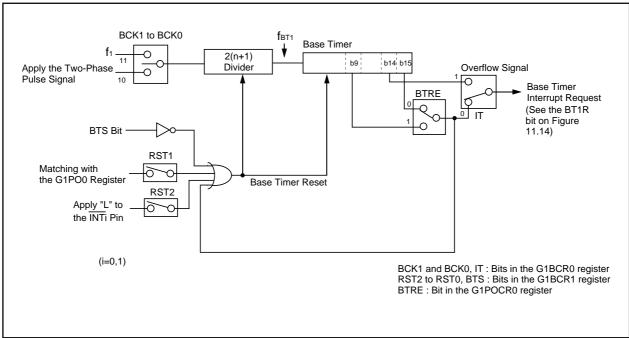
Figure 22.9 Base Timer Block Diagram
