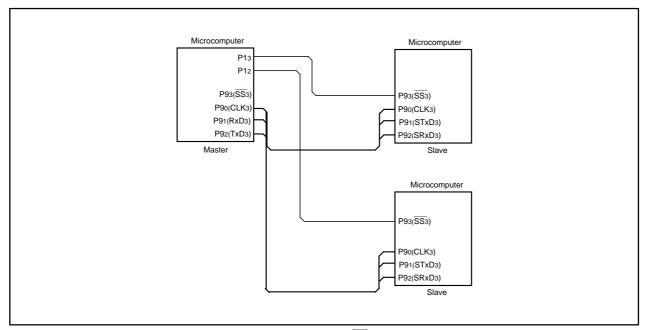
Figure 17.23 Serial Bus Communication Control with SS Pin
