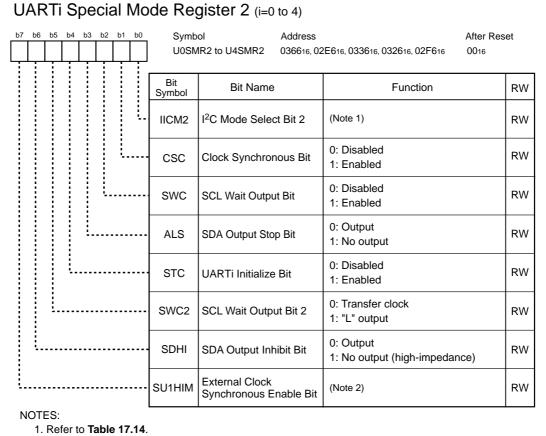
2. The external clock synchronous function can be selected by combining the SU1HIM bit and the SCLKDIV bit in the UiSMR register.
