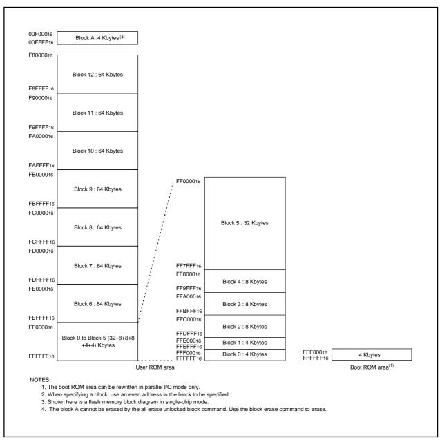
Figure 25.1 Flash Memory Block Diagram
