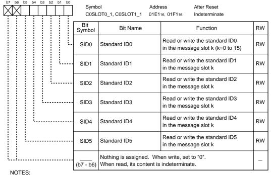
1. Select, by setting the C0SBS register, the message slot k to be accessed by the C0SLOTj\_1 register.
