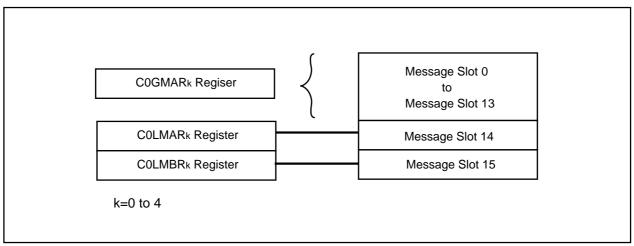
Figure 23.27 Mask Registers and Message Slots
