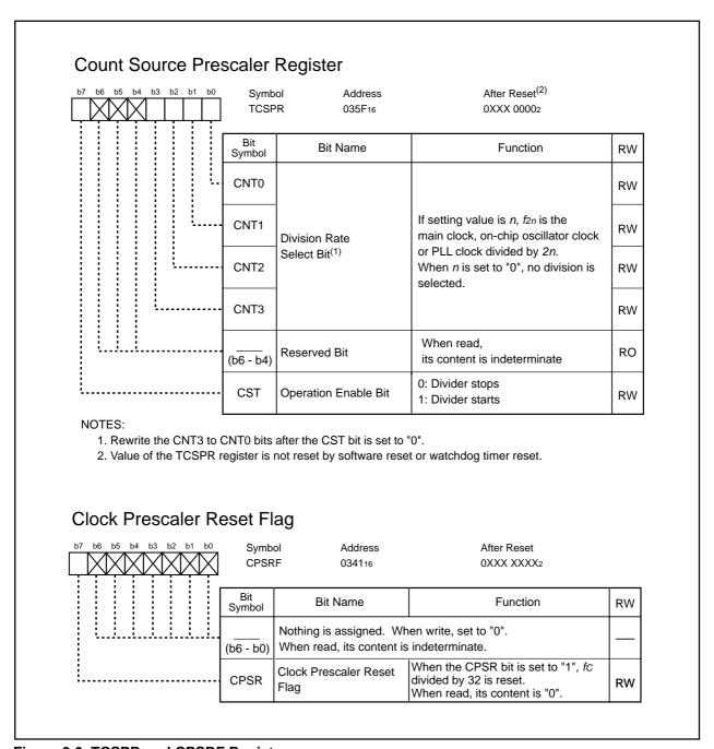
Figure 9.6 TCSPR and CPSRF Registers
