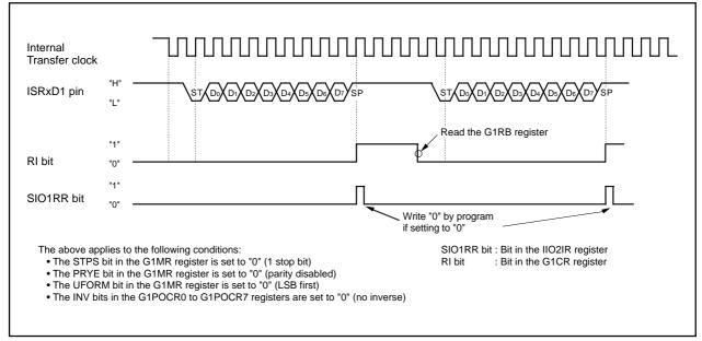
Figure 22.32 Receive Operation
