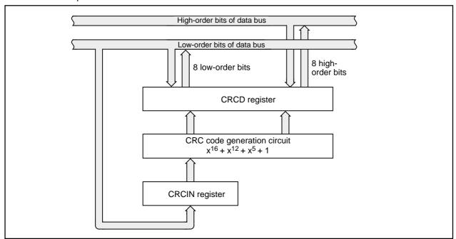
Figure 20.1 CRC Calculation Block Diagram
