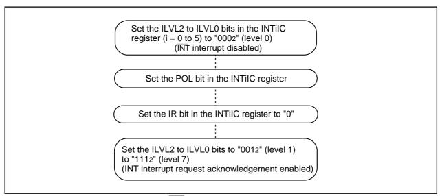
Figure 27.3 Switching Procedure for INT Interrupt
