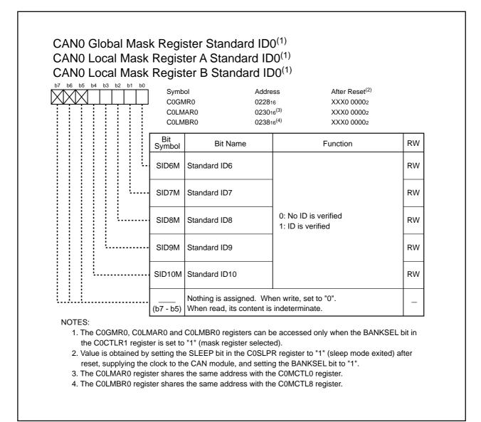
Figure 23.22 COGMR0, COLMAR0 and COLMBR0 Registers
