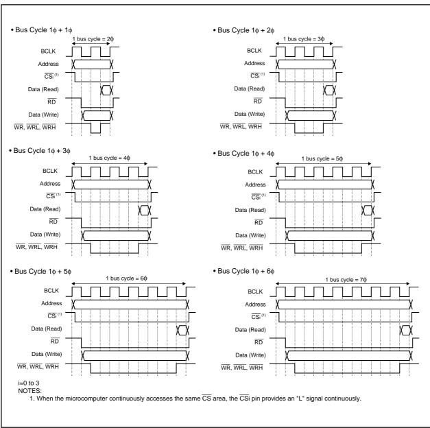
Figure 8.4 Bus Cycle with Separate Bus (1)
