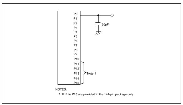
Figure 26.12 P0 to P15 Measurement Circuit
