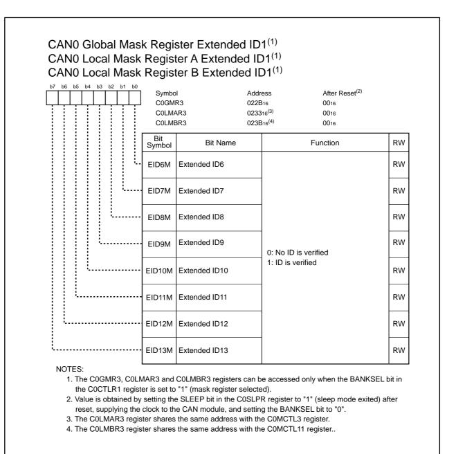
Figure 23.25 C0GMR3, C0LMAR3 and C0LMBR3 Registers
