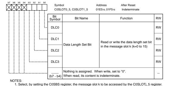
Figure 23.33 C0SLOT0\_4, C0SLOT1\_4, C0SLOT0\_5 and C0SLOT1\_5 Registers
