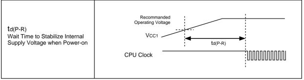
Figure 26.11 Power Supply Timing Diagram
