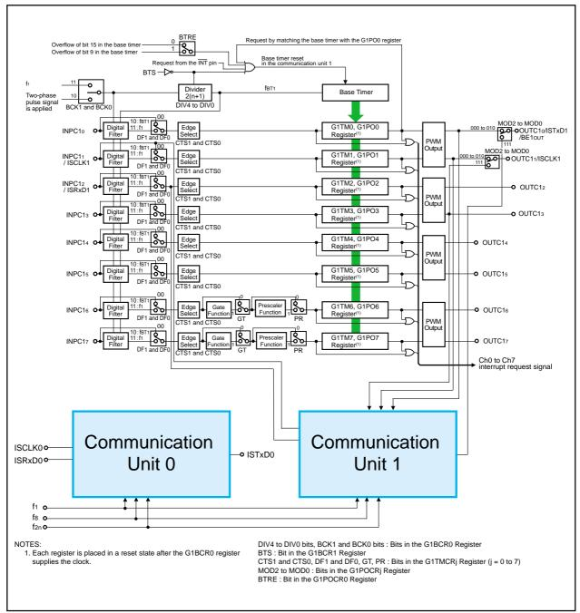
Figure 22.1 Intelligent I/O Block Diagram
