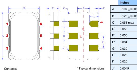
Gold 11.8 µinches 0.3 µm minimum over Nickel 50 to 350 µinches 1.27 to 8.89 µm
