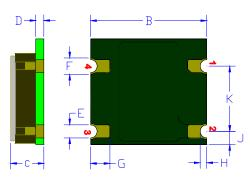
FR4 PCB Base: Solder masked All via holes tented on bottom Copper Clad ½ oz. Typical Gold plated 0.02 µinch (0.5 µm)
