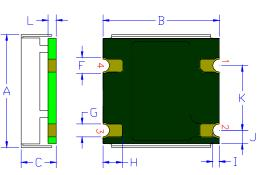
FR4 PCB Base: Solder masked All via holes tented on bottom Copper Clad ½ oz. Typical Gold plated 0.02 µinch (0.5 µm)
