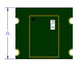
Label: Laser marked on the ceramic package metal cover
