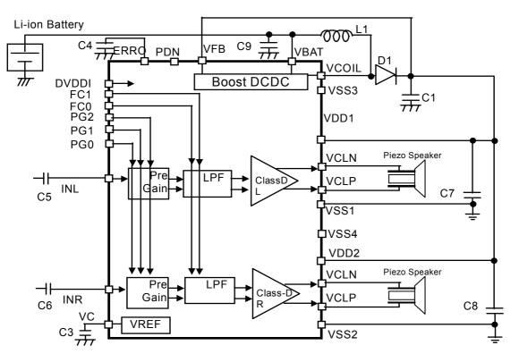
Figure 4 AK7846 Application Schematic
