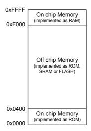
The figure below shows a typical Program Memories connections in system with DP8051CPU Microcontroller core.
