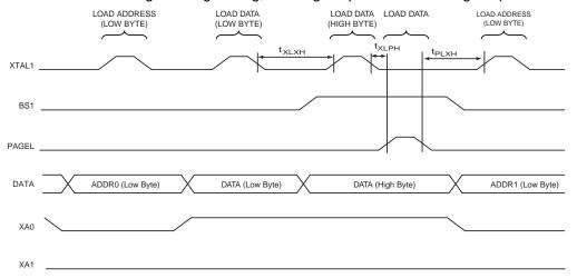
Note: 1. The timing requirements shown in Figure 28-7 (i.e., t<sub>DVXH</sub>, t<sub>XHXL</sub>, and t<sub>XLDX</sub>) also apply to loading operation.
