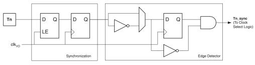
The synchronization and edge detector logic introduces a delay of 2.5 to 3.5 system clock cycles from an edge has been applied to the T1/T0 pin to the counter is updated.
