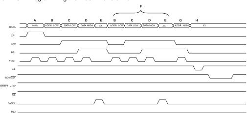
Figure 27-3. Programming the Flash Waveforms<sup>(1)</sup>
