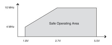
Figure 28-2. Maximum Frequency vs. V<sub>CC</sub>, ATmega48/88/168
