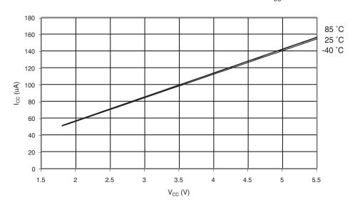
Figure 29-46. Analog Comparator Current vs.  $V_{\rm CC}$
