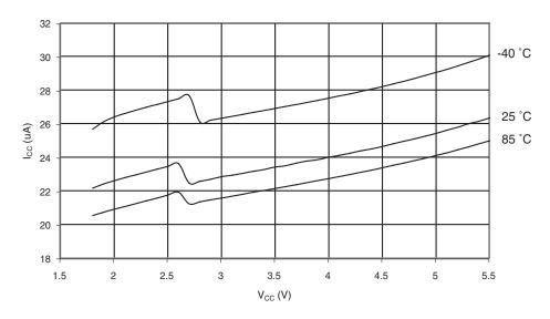
Figure 29-44. ADC Current vs.  $V_{CC}$  (AREF =  $AV_{CC}$ )
