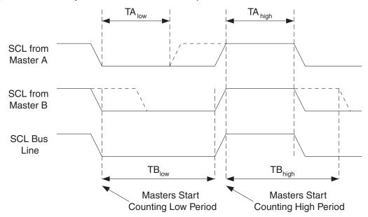
Figure 21-7. SCL Synchronization Between Multiple Masters
