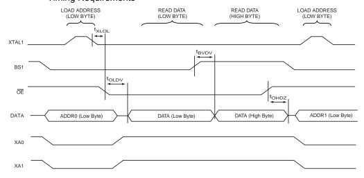
Note: 1. The timing requirements shown in Figure 28-7 (i.e., t<sub>DVXH</sub>, t<sub>XHXL</sub>, and t<sub>XLDX</sub>) also apply to reading operation.
