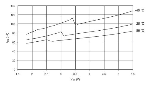
Figure 29-47. Programming Current vs. V<sub>CC</sub>
