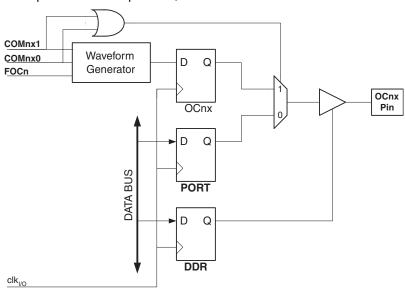
Figure 14-4. Compare Match Output Unit, Schematic
