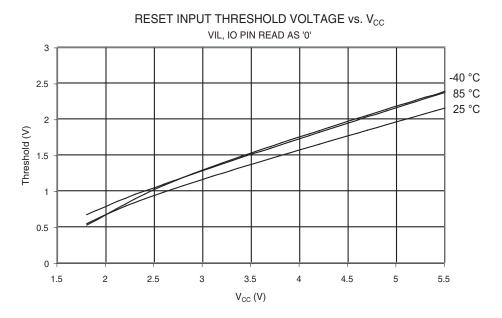
Figure 29-32. Reset Input Pin Hysteresis vs.  $V_{\rm CC}$
