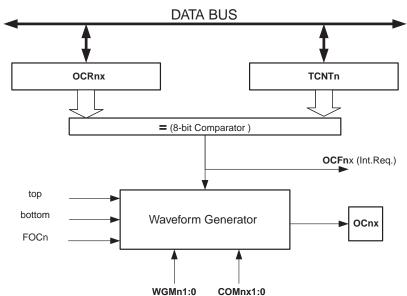
Figure 14-3. Output Compare Unit, Block Diagram
