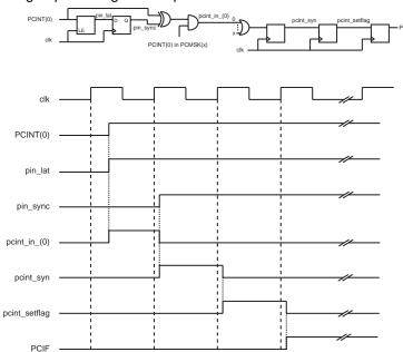
Figure 12-1. Timing of pin change interrupts
