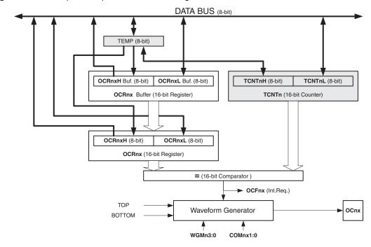
Figure 15-4. Output Compare Unit, Block Diagram
