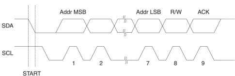
Figure 21-4. Address Packet Format
