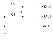
The Low Power Oscillator can operate in three different modes, each optimized for a specific frequency range. The operating mode is selected by the fuses CKSEL3..1 as shown in Table 8-3 on page 31.
