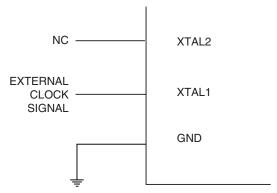
When this clock source is selected, start-up times are determined by the SUT Fuses as shown in Table 8-13.
