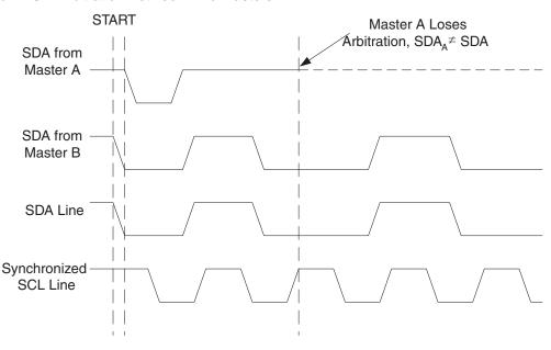
Figure 21-8. Arbitration Between Two Masters
