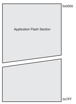
**Figure 7-2.** Program Memory Map, ATmega88 and ATmega168
