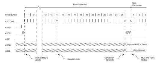
Figure 23-5. ADC Timing Diagram, Single Conversion
