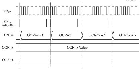
Figure 15-11. Timer/Counter Timing Diagram, Setting of OCF1x, with Prescaler (f<sub>clk I/O</sub>/8)
