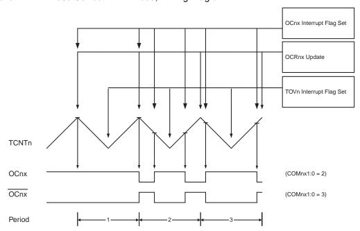
Figure 17-7. Phase Correct PWM Mode, Timing Diagram
