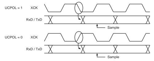
The UCPOLn bit UCRSC selects which XCKn clock edge is used for data sampling and which is used for data change. As Figure 19-3 shows, when UCPOLn is zero the data will be changed at rising XCKn edge and sampled at falling XCKn edge. If UCPOLn is set, the data will be changed at falling XCKn edge and sampled at rising XCKn edge.
