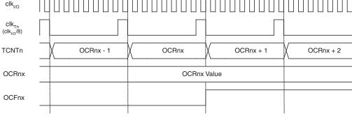
Figure 14-11 shows the setting of OCF0A and the clearing of TCNT0 in CTC mode and fast PWM mode where OCR0A is TOP.
