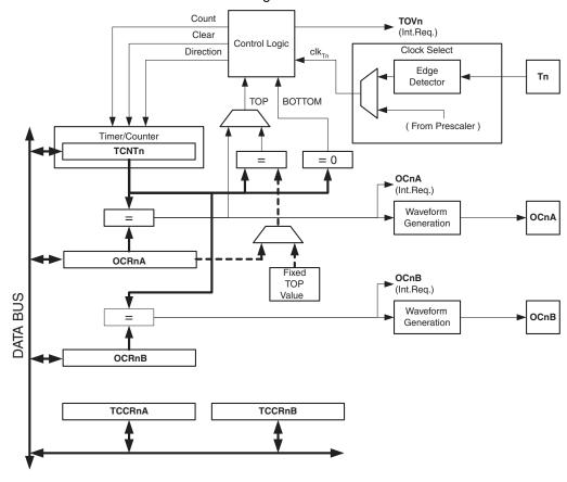
Figure 14-1. 8-bit Timer/Counter Block Diagram
