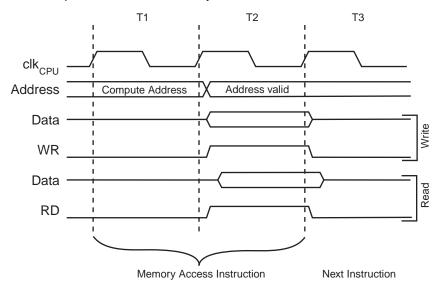
Figure 7-4. On-chip Data SRAM Access Cycles
