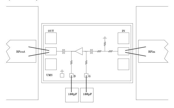
Note: Supply feed should be capacitively bypassed. 25µm diameter gold wire is to be prefered.
