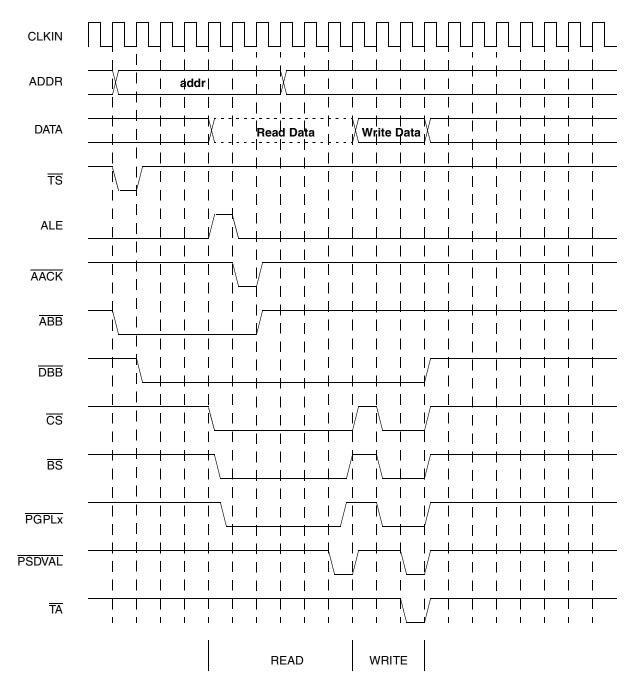
Figure 9. UPM with Read-Modify-Write Cycle
