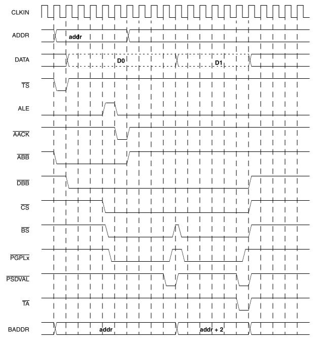
Figure 2 shows a 32-bit single beat read/write on a 16-bit port.
