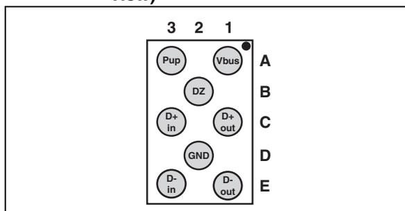
**Figure 2. Schematic**
