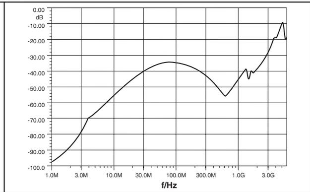
Figure 5. ESD response to IEC61000-4-2 (+15 kV air discharge) on one input V(in) and on one output (Vout)
