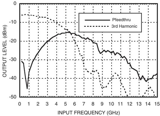
**Reverse Leakage, Pin= 0 dBm, T= 25 °C**
