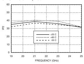
Input IP2 vs. Temperature @ LO = -5 dBm, Vdd = +3V \*
