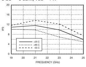
Input IP3 vs. Temperature @ LO = -5 dBm, Vdd = +3V \*
