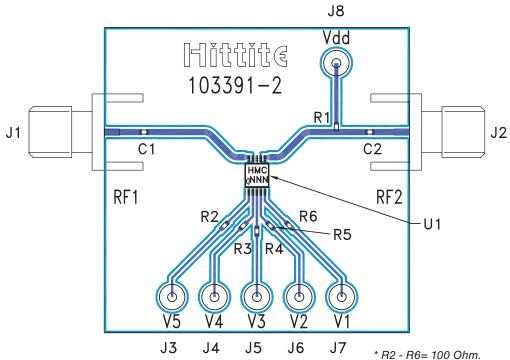
These resistors are optional and may be used to enhance decoupling of the RF path from the control inputs.
