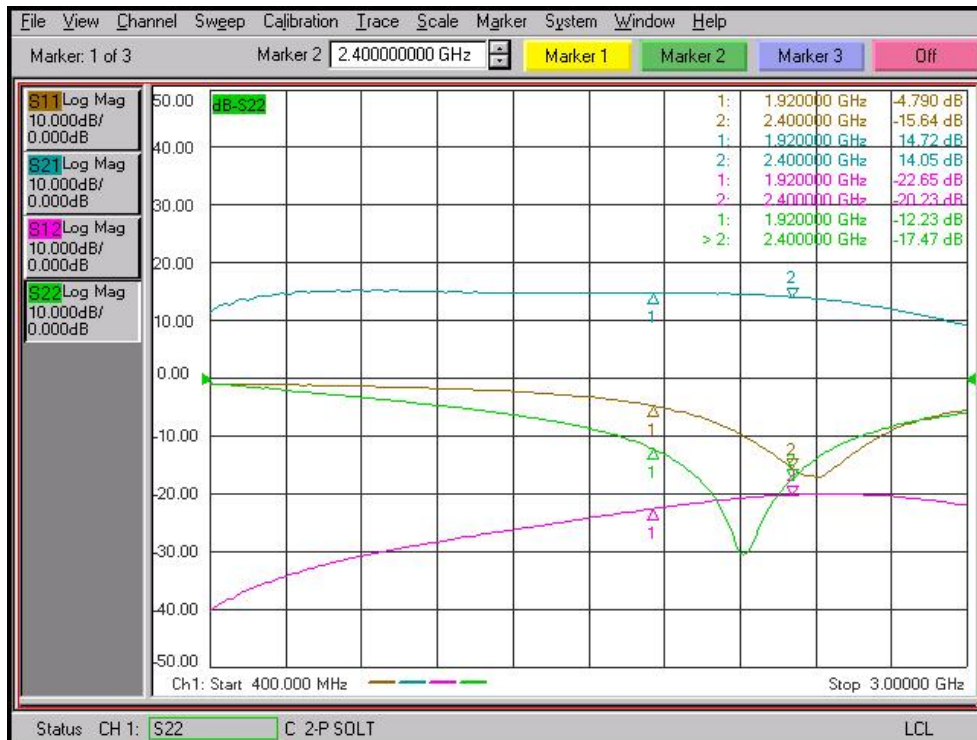
Figure 138. S22 and S11 Matching for ADL5521, 2.4GHz Example
