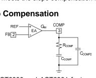
The ACT6390 and ACT6391 feature a simple loop compensation scheme. Simple follow the procedure detailed below to determine suitable compensation components. For best results be sure to prototype to confirm the values, and adjust the compensation network (by inspecting the transient response, for example) as needed to optimize results for your particular application.
