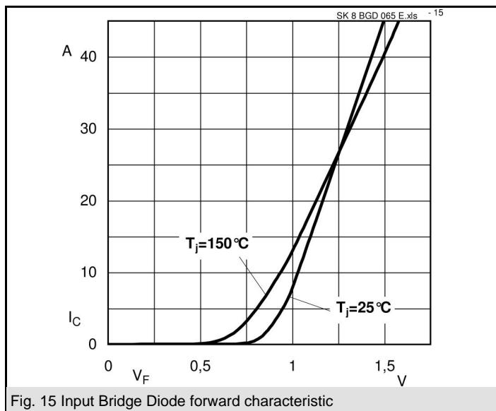
Fig. 15 Input Bridge Diode forward characteristic
