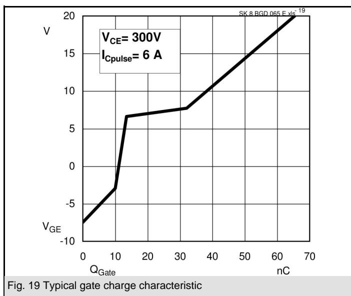
Fig. 19 Typical gate charge characteristic
