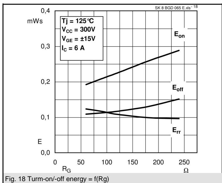
Fig. 18 Turn-on/-off energy =  $f(R_g)$
