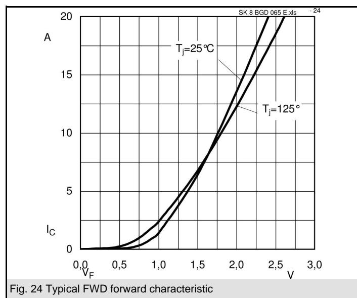
Fig. 24 Typical FWD forward characteristic
