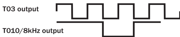
b) Pulse non-inverted, Reg.7A[3:2] = 01
