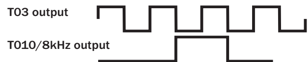
d) Pulse inverted, Reg.7A[3:2] = 11
