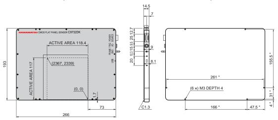
Top cover material including window is carbon fiber (1.0 mm thickness). Weight: 1.2 kg
