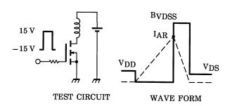
$$\begin{aligned} &R_G = 25~\Omega \\ &V_{DD} = 90~V,~L = 8.3~mH \end{aligned} \qquad EAS = \frac{1}{2} \cdot L \cdot I^2 \cdot \left( \frac{BVDSS}{BVDSS - VDD} \right) \end{aligned}$$
