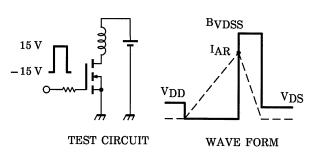
$R_G = 25 \ \Omega$  $EAS = \frac{1}{2} \cdot L \cdot I^2 \cdot \left(\frac{BVDSS}{BVDSS - VDD}\right)$  $V_{DD}$  = 25 V, L = 398  $\mu H$
