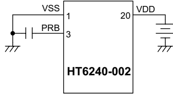
Fig. 13 Example of power-on reset function
