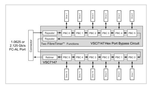
Several VSC7147's can be cascaded together to create a JBOD. The flexibility of the FibreTimers allow repeater and retimer functions to reside where they make the most sense for the backplane board design.
