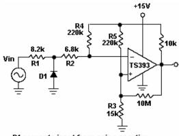
D1 prevents input from going engative by more than 0.6V, R1 + R2 = R3 R3 <= R5 / 10 for small error in zero crosing
