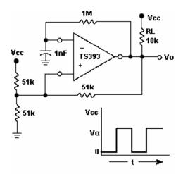
Figure 6. free-running square-wave oscillator
