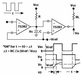
Figure 7. time delay generator
