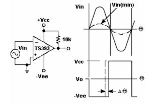
Vin(min)=0.4V peak for 1% phase distortion (∆ 8)
