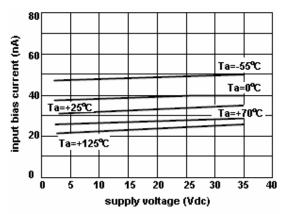
Figure 1. input bias current vs power supply voltage
