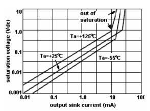
Figure 2. output saturation voltage vs output sink current
