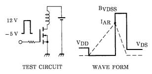
$$\begin{array}{l} T_{ch} = 25^{\circ}C \; (Initial) \\ Peak \; I_{AR} = 5 \; A, \; R_G = 25 \; \Omega \\ V_{DD} = 16 \; V, \; L = 1.0 \; mH \end{array} \\ \to E_{AS} = \frac{1}{2} \cdot L \cdot I^2 \cdot (\frac{B_{VDSS}}{B_{VDSS} - V_{DD}})$$
