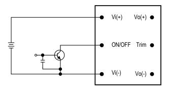
Figure 17: Circuit configuration for remote ON/OFF
