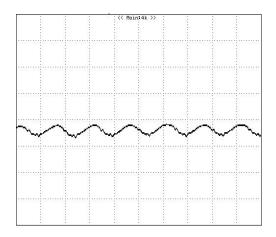
**Figure 9**: Input reflected ripple current,  $i_{\rm S}$ , at full rated output current and nominal input voltage with 12 $\mu$ H source impedance and 68 $\mu$ F electrolytic capacitor (20 mA/div).
