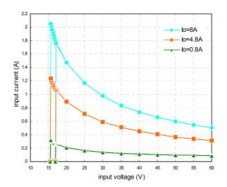
Figure 3: Typical input characteristics at 25°C.
