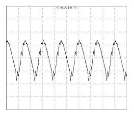
**Figure 11:** Output voltage ripple at nominal input voltage and rated load current (20 mV/div). Load capacitance: 1μF ceramic capacitor and 10μF tantalum capacitor. Bandwidth: 20 MHz.
