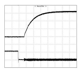
**Figure 4:** Turn-on transient at full load current (Constant resistance mode) (1 ms/div). Vin: 48V; Top Trace: Vout (1V/div); Bottom Trace: ON/OFF Control (5V/div).
