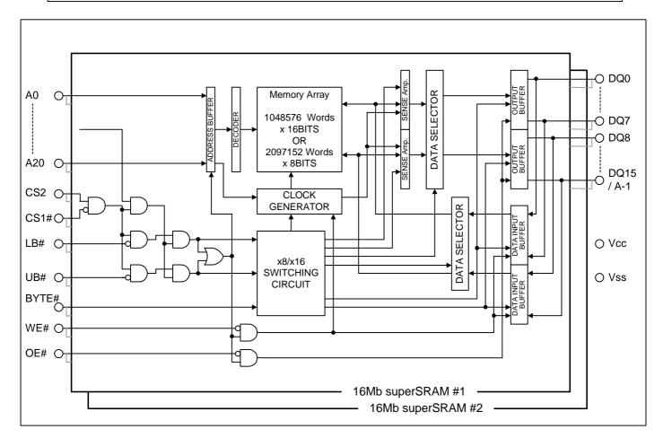
Note: BYTE# pin supported by only TSOP type.
