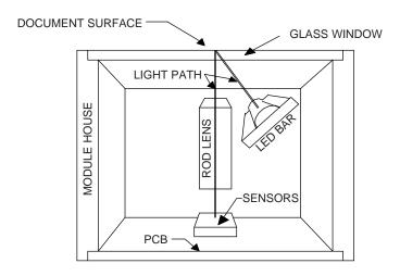
INSIDE PICTORIAL OF MODULE Figure 1. PI225MC-A6 Cross Section
