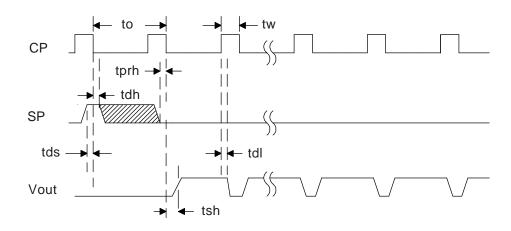
MODULE TIMING DIAGRAM
