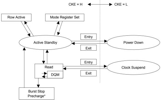
\* All operation of "Precharge" command is to stop burst read.
