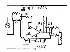
When a true common ground point cannot be used, a heavy ground conductor or ground plane should be used.
