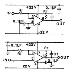
The use of a feedback capacitor, Cf, cancels the input capacitance of the integrated circuit, and the wiring capacitance at the summing junction. Typical values of Cf are 3-10pF.
