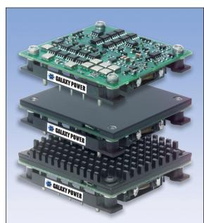
The open-frame Taurus HC is also available with a heat-spreading baseplate or complete with an optional heatsink.
